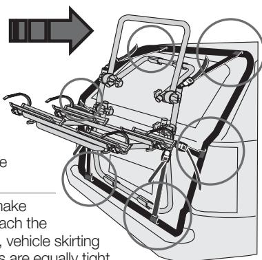
**EN** Attach the fastening straps to the vehicle's rear door and make sure that each part of the door is made of metal. Do not attach the fastening straps to plastic parts such as bumpers, spoilers, vehicle skirting or any other kind of plastic part. Pay attention that all straps are equally tight.
